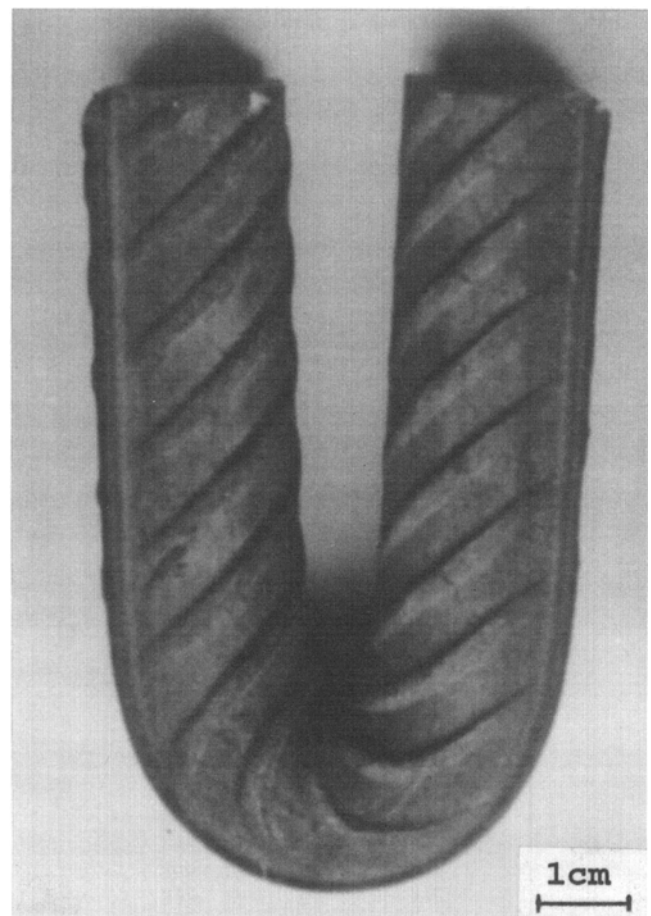
Fig. 6 Photograph of close bend obtained in a 20 mm diam Cu-Cr-TMT rebar (550 MPa YS grade) showing no manifestation of surface cracks
